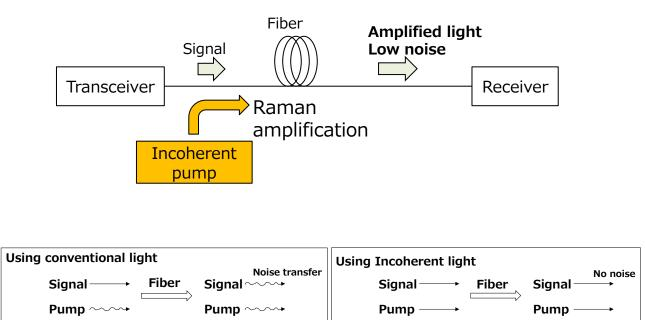
Fig. 1: Schematic diagram of forward Raman amplification
