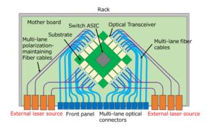
Fig. 1 Schematic top view of network switch server employing CPO
